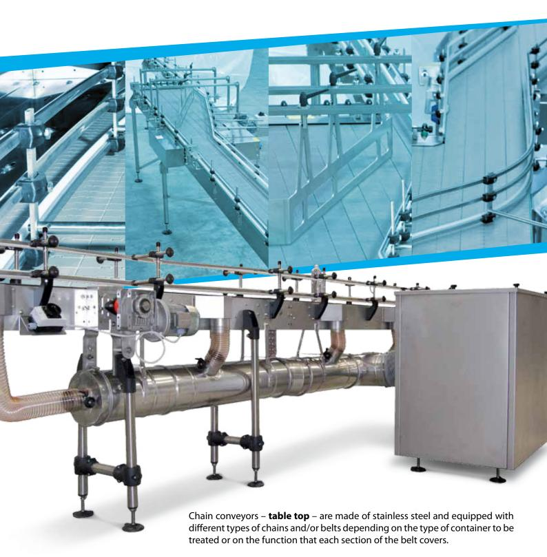
In case it is necessary to carry empty and particularly unstable containers, it is possible to equip our table top conveyors with a vacuum assisted device in order to increase stability.
